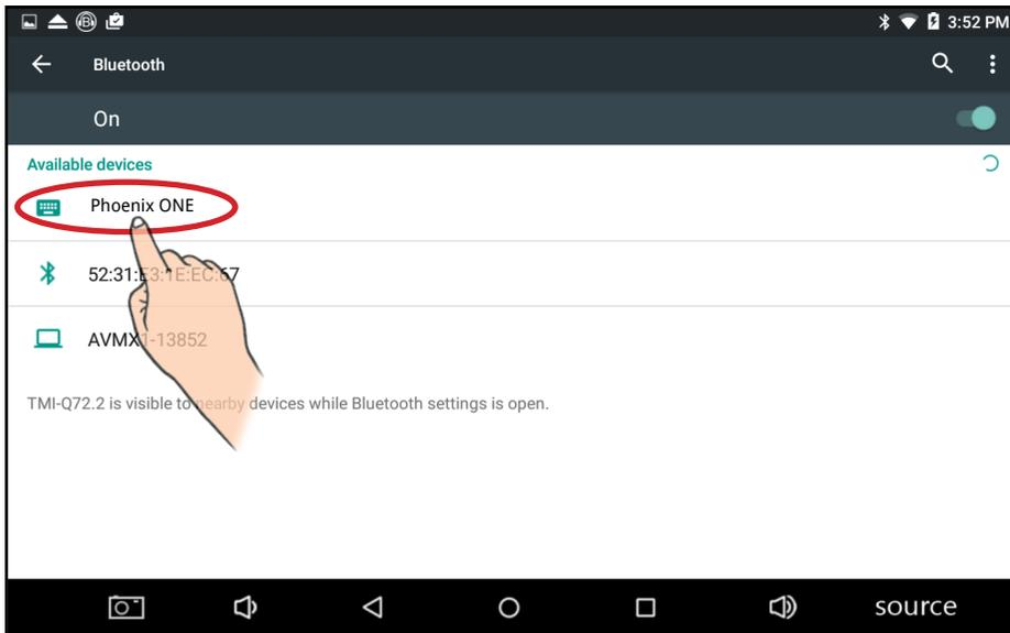
5. Once the controller is in Pairing mode, search for the device (Phoenix ONE/MINI) on the Tablets Bluetooth screen.
