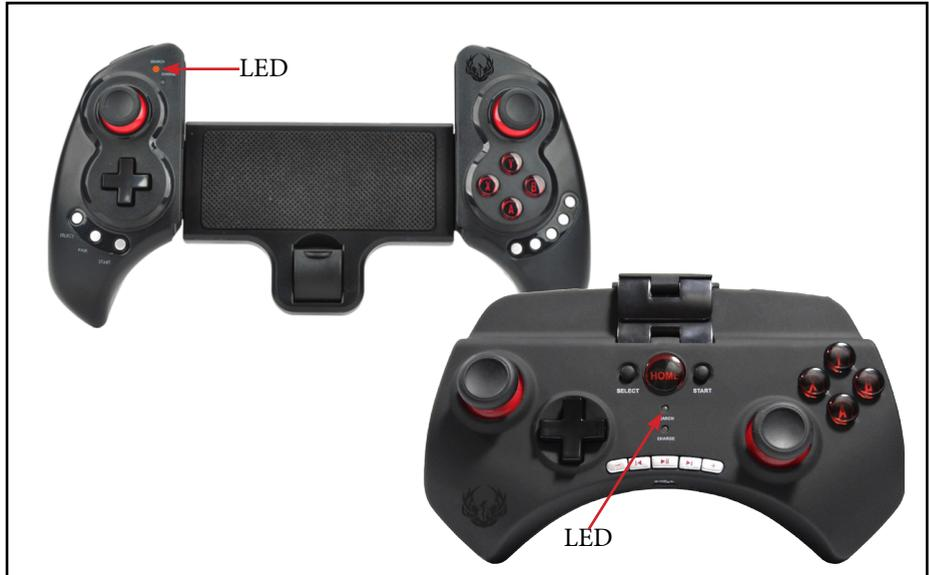
8. Once the controller is connected the LED light will stay lit.
