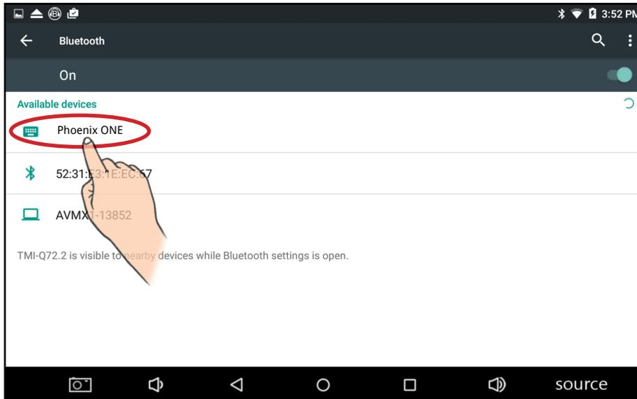
1. Once the controller is in Pairing mode, search for the device (Phoenix ONE or Phoenix MINI) on the Tablets Bluetooth screen.
