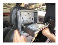
6. Close the door to the "carrier bucket." Make sure there is nothing preventing the bucket from opening or closing securely.
