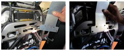
2. Using the provided hardware, loosely mount the seatback bracket to the seat frame.
