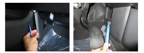
3. Remove the lower side panels of the center console exposing the 10mm screws on the back side of the center console. Remove all silver screws on the back of the console in order to remove the back of the center console.
