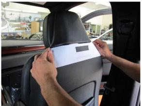
3. Carefully mark the cut location on the vehicle's seat back.
