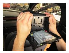
5. Firmly press the "carrier bucket" into headrest. Please pay special to the side of the bucket as they need to be squeezed firmly to engage the locking clips.
