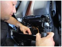
Located behind the center console is the cigarette lighter socket. Using a voltmeter, test both cables going into cigarette lighter for your ground.
