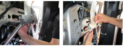
3. Once the bracket has been loosely mounted and centered, you can begin the final tightening of the screws.
