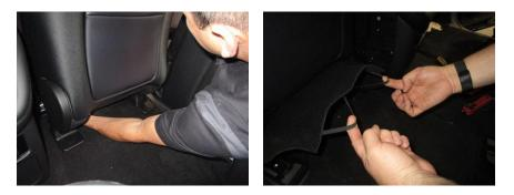
5. Using a plastic panel tool, carefully unclip the front of seatback from the rear seatback.
