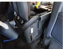
4. After opening the center console, firmly grip the side on the back of the center console and pull towards the rear of the vehicle. (Note: Make sure to be gentle in order to not damage or lose any clips.)
