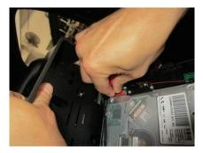
Loop the post cables and clip them into the post cables clips located on either side of the DVD player. (Note: Pay special attention to the photos below on how high to have the cables and how the cables need to be twisted. If performed incorrectly cable will prevent the bucket from closing, continuously eject the DVD, or fail to let the DVD play.)
