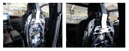
2. Follow the seat's factory wiring to run the post cables down under the seat.
