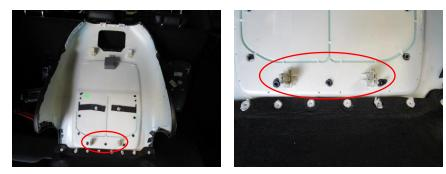
7. Grip both sides of the seatback and carefully pull the seatback towards you and downward. (Note: There are 2 clips that are located at the bottom of the headrest panel that point downward. When removing the seatback, be mindful of their location.)
