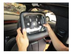
2. Using the provided screws, mount the "back plate" to the "seatback bracket" and pull the wires through as shown below.
